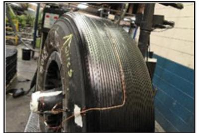
**Press and mold type will dictate how the thermocouple wires can be handled in order to properly exit the mold.**
