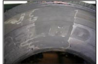
8. Gather all of the thermocouple wires midway down the sidewall. If desired, cover the wires with calendered cushion gum up to the point where they emerge from the tread and stitch down. Other means to hold the wires in place may also be used as long as the wires are not damaged in the process.
