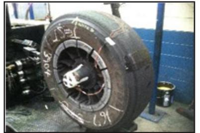
8. Apply the tread rubber to the buffed casing using the specific program for the mold to be used. Monitor the tread rubber application to ensure the thermocouple wires do not become loose during the process.
