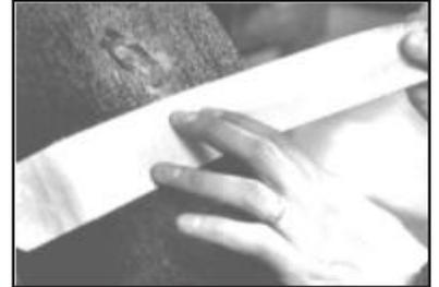
**Masking tape should be used over other tapes such as duct tape because it will not melt under the elevated mold temperatures.**
