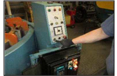
6. Carefully guide the thermocouple wires or cable between the segments while the press is closing to ensure the wires are in between the shims and not pinched at the segment split.
