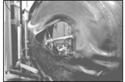
4. With the tire now on the bottom rim half, bring the thermocouple wires to the tube stem (stem now protruding through the slot in the rim) and tape them to the stem.
