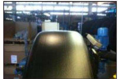
3. For ease of handling, cut a piece of precure tread in your selected pattern approximately 24" (610mm) in length on which to place the thermocouple wires. If desired, a full length tread may be used.
