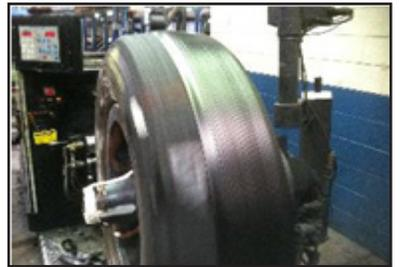
9. After the tread rubber has been applied, place a final thermocouple wire on top of the rubber at the location of the other thermocouple wires to record the temperature of the mold matrix. Run the wire down the tire and out with the other thermocouple wires.
