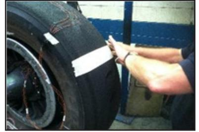
6. Apply black cement to the masking tape with a stipple brush and allow to dry. The extruded tread rubber will not adhere to the tape when building if it is not cemented.
