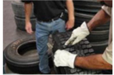
10. Check the tread cross section for proper undertread gauge (4/32-5/32" (3-4mm)) and for any porosity. If porosity did occur, the cure was not complete and the thermocouple study will need to be rerun once the mold has cooled.
