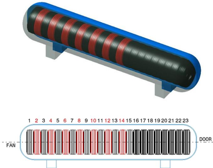
Figure A. Thermocouples on tires indicated in red - 23 tire previously tested chamber
