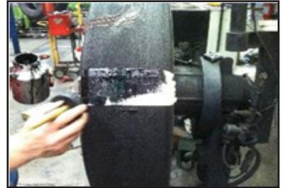
**A cable can be made of the various wires. Holding them together with tape will make the thermocouple wires more manageable (use small pieces of masking tape spacing them approximately 12" (30cm)).**
