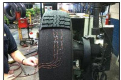
4. Continue this process until all thermocouple wires are placed and properly secured. Remove the mold cure tread cut-out from the buffed casing.
