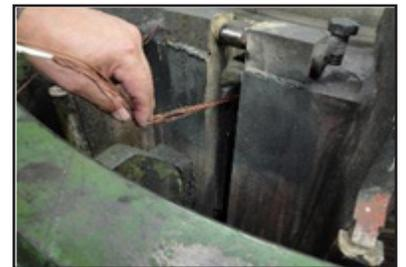
7. Use a data collection sheet to take readings on a regular interval of time. Readings should continue until the correct number of cure equivalents has been reached. Continue to take a few more readings beyond the point where the cure equivalents has been obtained.
