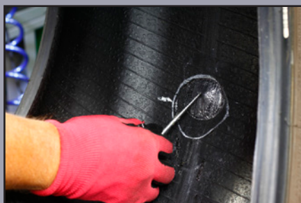
Press Repair Unit into Place
