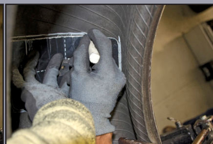
Trace Around Repair Unit Template
