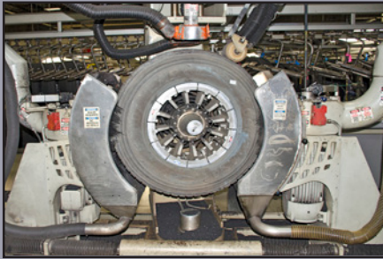
Casing on a Buffing Machine
