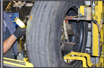
Inspect Outside of Casing
