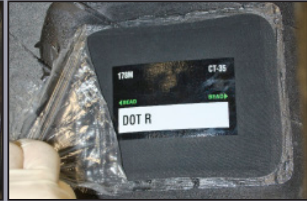
Remove Film from Repair Unit
