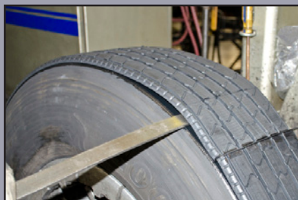
Match Tread Pattern at the Splice
