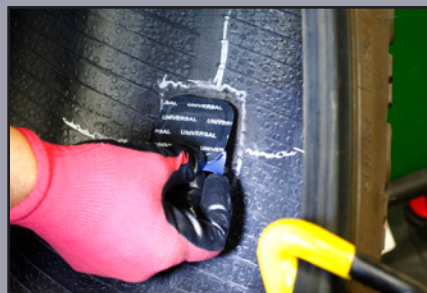
Install the Repair Unit
