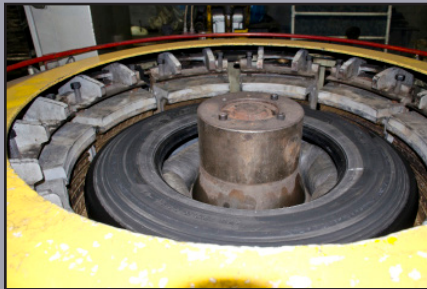
Casing in Tire Curing Press
