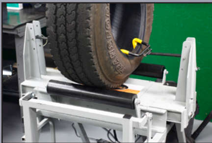
Place Tire on Inspection Machine
