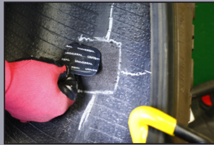
Two Piece Repair Unit
