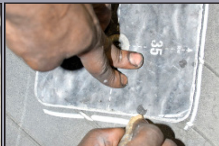
Trace Around Repair Unit
