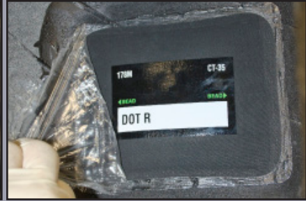
Remove Film from Repair Unit
