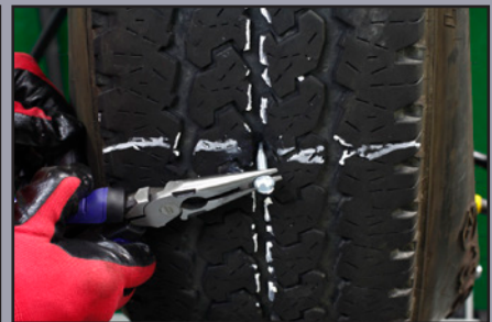
Remove Penetrating Object
