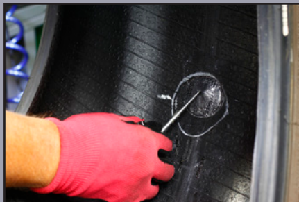
Press Repair Unit into Place
