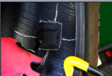
Apply Repair Sealant
