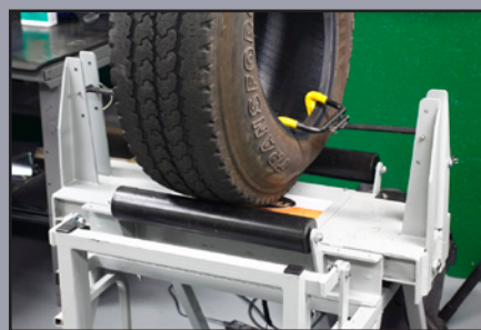
Tire Casing on Inspection Machine
