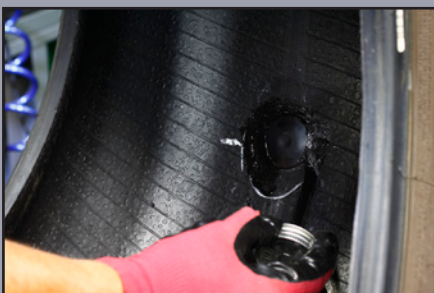
Apply Repair Sealant
