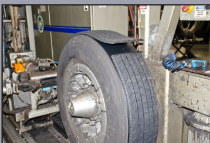
Cut Tread Ends to Proper Length
