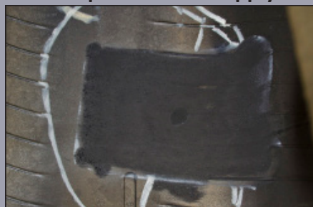
Repair Area After Filling and Buffing
