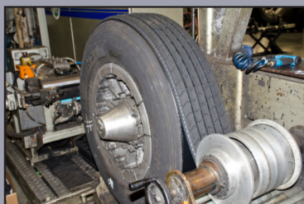
Apply Tread to Buffed Casing
