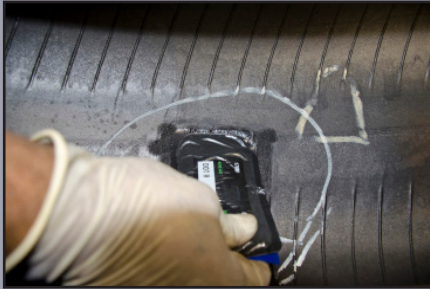
Install Repair Unit
