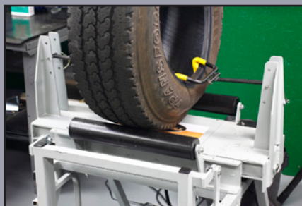
Tire Casing on Inspection Machine
