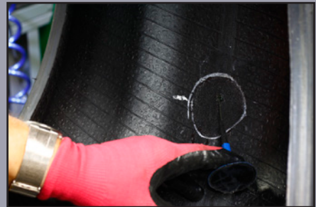
Install the Repair Unit
