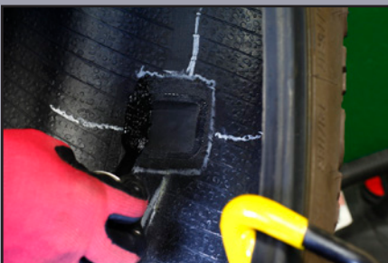
Apply Repair Sealant
