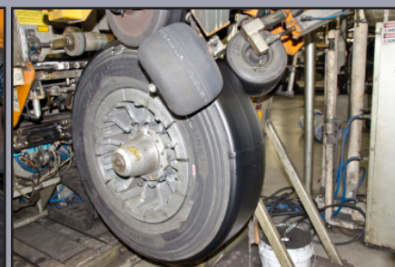
Apply Rubber to Buffed Casing
