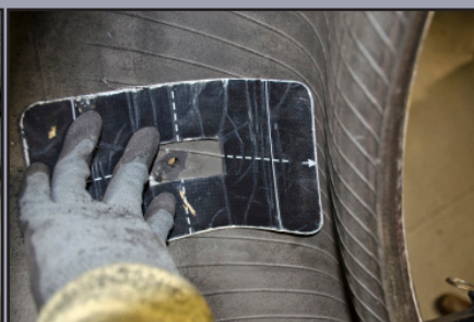
Measure for Repair Unit
