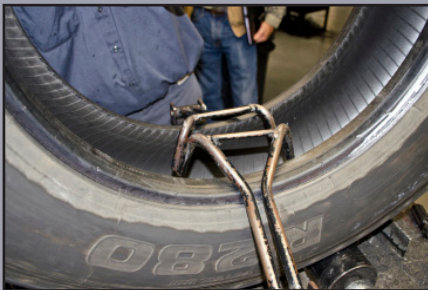
Spread Beads for Inspection
