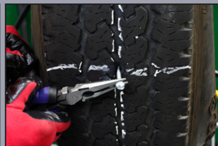
Remove Penetrating Object
