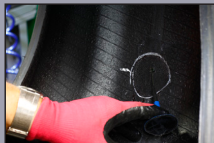
Install the Repair Unit
