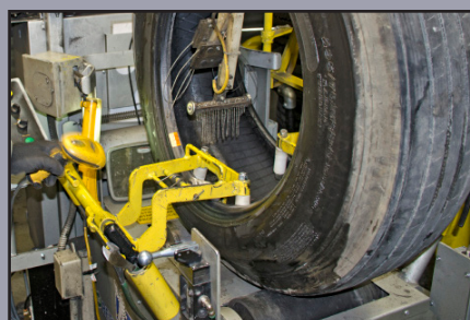
Tire Casing on Inspection Machine
