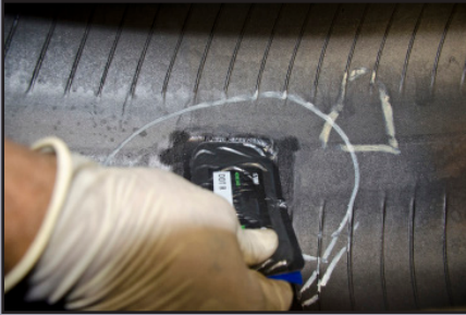
Install Repair Unit
