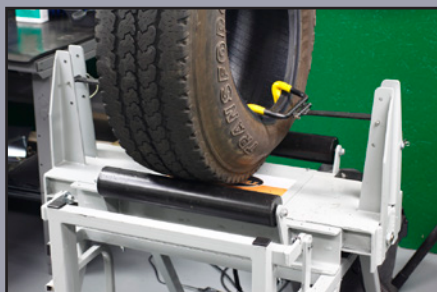
Place Tire on Inspection Machine
