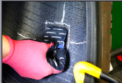
Install the Repair Unit
