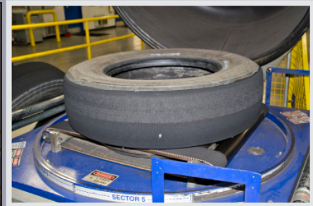
Casing on Shearography Machine
