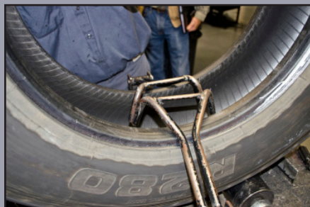
Spread Beads for Inspection
