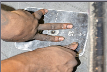
Measure for Repair Unit
