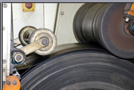
Apply Rubber to Buffed Casing
