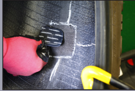
Two Piece Repair Unit
