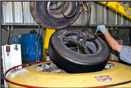
Place Casing in Tire Curing Press
