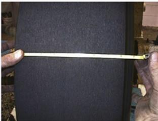
Checking for Proper Buffed Width
