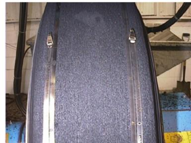
Be sure that shoulders are of equal height and that the tires are buffed completely over the area to be covered by the new full
